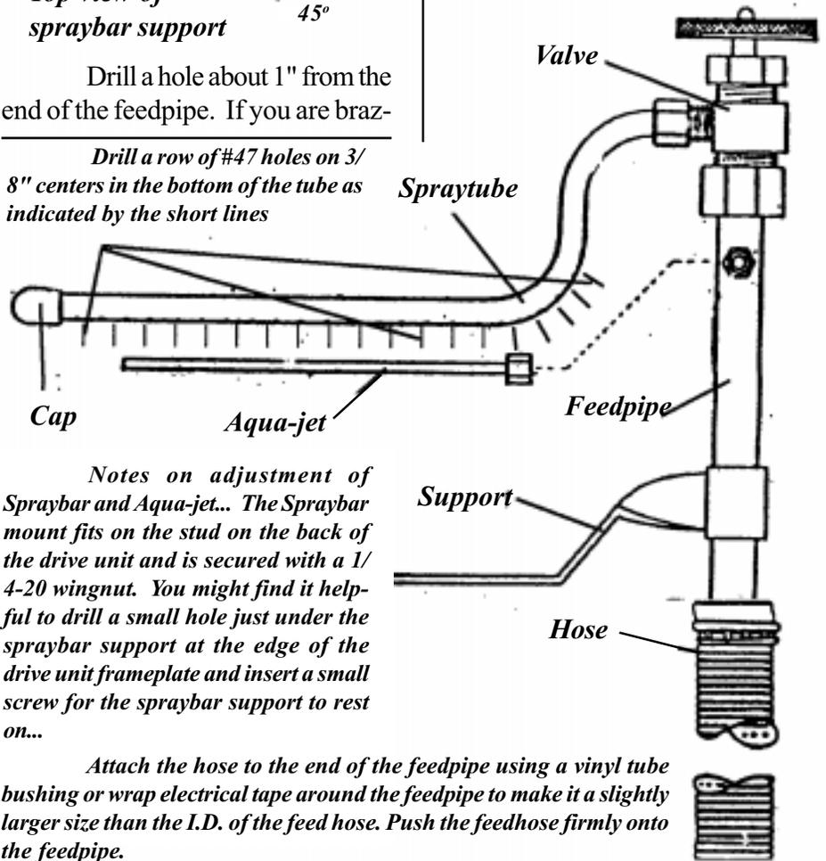
Notes on adjustment of Spraybar and Aqua-jet... The Spraybar mount fits on the stud on the back of the drive unit and is secured with a 1/4-20 wingnut. You might find it helpful to drill a small hole just under the spraybar support at the edge of the drive unit frameplate and insert a small screw for the spraybar support to rest on...
