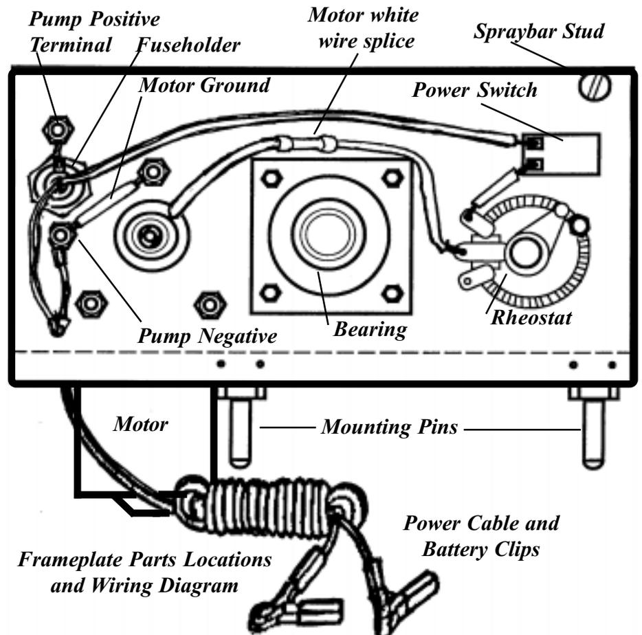
**Frameplate Parts Locations and Wiring Diagram**
