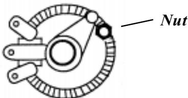
Using a small amount of epoxy, glue a small nut to the surface of the Rheostat to prevent it being turned beyond the 15 RPM mark. Be very careful not to get any epoxy on the rheostat wiper and set the drive unit
