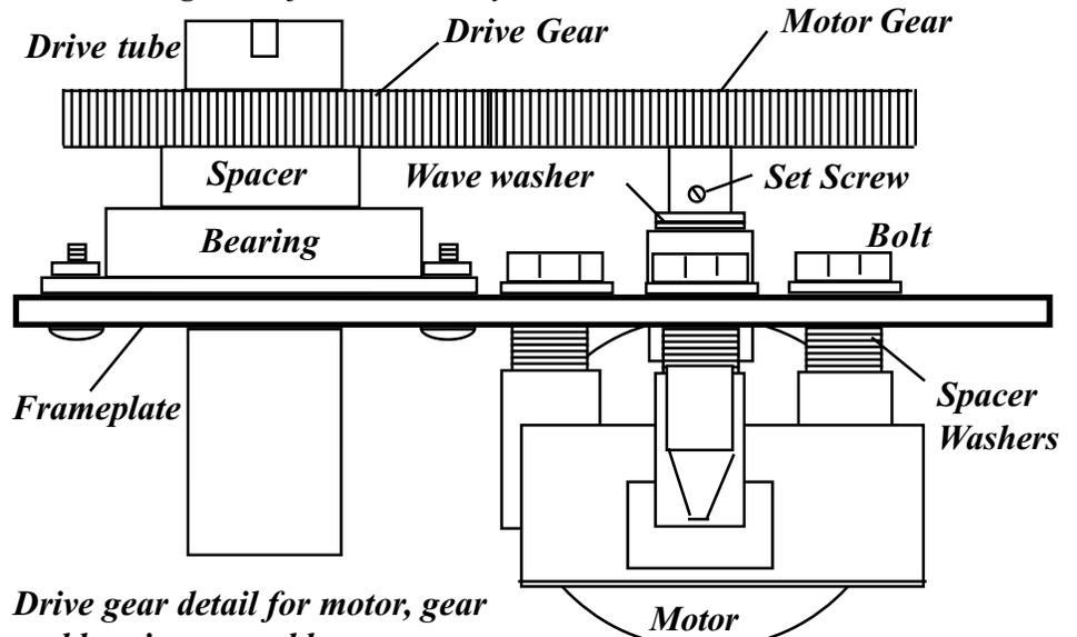
**Drive gear detail for motor, gear and bearing assembly.**
