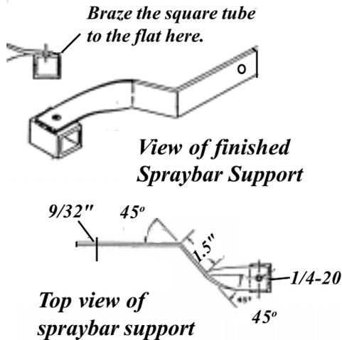
Drill a hole about 1" from the end of the feedpipe. If you are brazing
